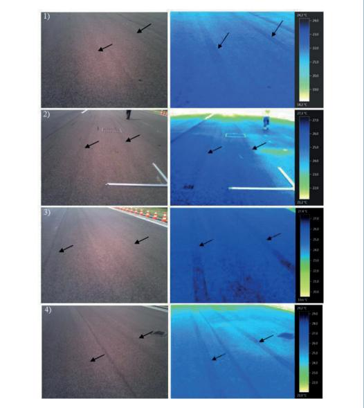
Fig. 2. Thermal image of skid mark [6]
